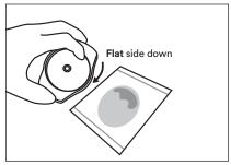
With **flat** side down, place 3M<sup>™</sup> Petrifilm<sup>™</sup> Spreader on top film over inoculum.
