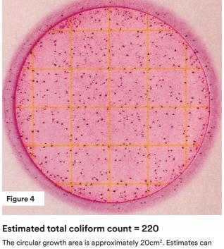
The circular growth area is approximately 20cm². Estimates can be made on plates containing greater than 150 colonies by counting the number of colonies in one or more representative squares and determining the average number per square. Multiply the average number by 20 to determine the estimated count per plate.
