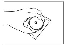
Gently apply pressure on Petrifilm spreader to distribute inoculum over circular area before gel is formed.
