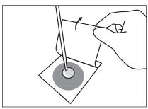
Place 3M™ Petrifilm™ Coliform Count Plate on level surface. Lift top film. With 3M™ Electronic Pipettor or equivalent held perpendicular to plate, place 1mL of sample or diluted sample onto center of bottom film.
