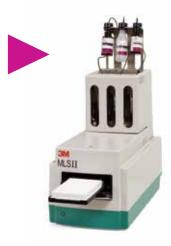
Step 2: Place micro-plate into the MLS instrument and select the appropriate assay.
