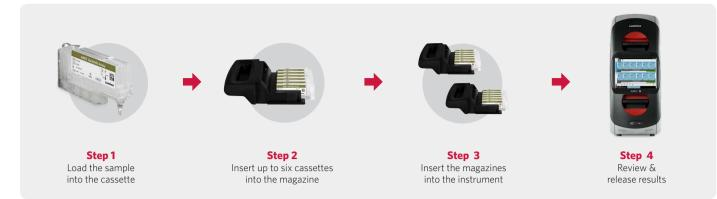
The operator simply adds specimen to the sample chamber, puts the cassette in the magazine, loads the magazine into the ARIES<sup>®</sup> System, and the run will start automatically.
