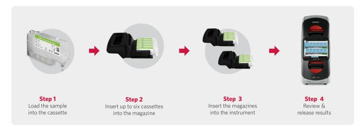
The operator simply adds specimen to the sample chamber, puts the cassette in the magazine, loads the magazine into the ARIES® System, and the run will start automatically.
