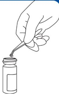
Aseptically remove 1 pellet with sterile forceps from the vial. Do not remove desiccant.
