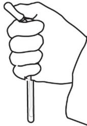
Break red snap valve at the top of the UV-BioTAG swab to release the hydrating fluid.
